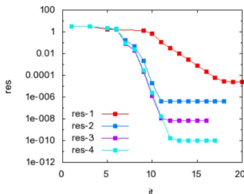
residuals level off at error of time integration = perturbation level of measurements
