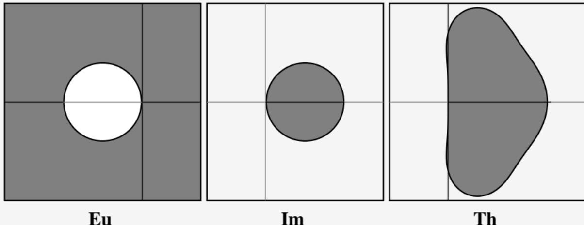
The Euler method has very poor stability and it should not be used with stiff problems.
