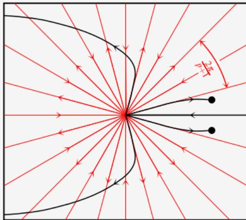
For an A-approximation, we must avoid an arrow diagram like the following, because we cannot have an up-arrow from zero crossing the imaginary axis on its way to  $-\infty$ .
